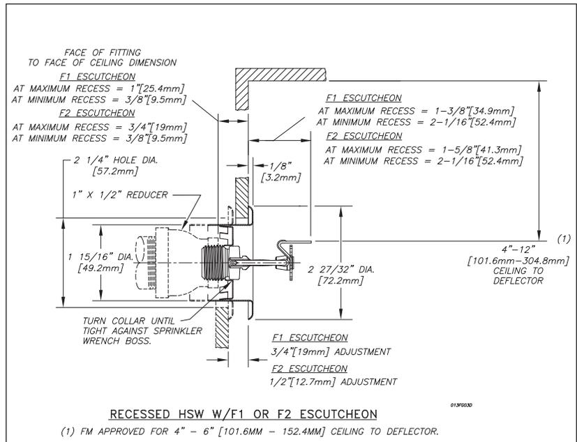
**Note:** For Recessed HSW Sprinklers use installation wrench W4. FM and cULus permits use with F1 or F2 escutcheons for "Light Hazard" only.
