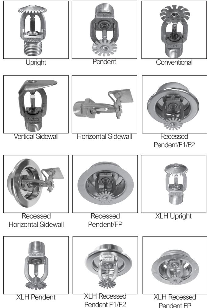
The F156, F142, F1XLH & F128 Series Automatic Sprinkler utilizes a 5.0 mm frangible glass bulb. The glass bulb consists of an accurately controlled amount of special fluid hermetically sealed inside a precisely manufactured glass capsule. This glass bulb is specially constructed to provide fast thermal response.
