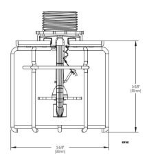
**Note:** When using the S-5 Water Shield with the Model 22 Guard, the S-5 Water Shield replaces the locking nut shown.
